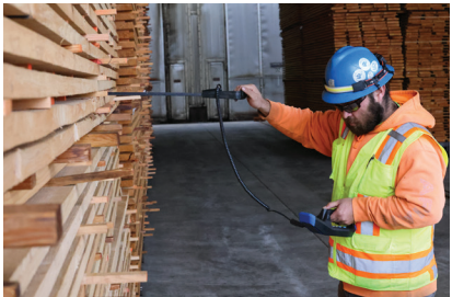
THE L5300 PAIRED WITH THE L722 STACK PROBE DIVES DEEP INTO LUMBER STACKS TO UNCOVER HIDDEN MOISTURE
