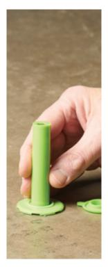
After the initial equilibration has been reached per ASTM F2170 requirements, subsequent readings can be taken instantly. If future testing is needed, replace the protective plug by pushing it back into the protective cap.
